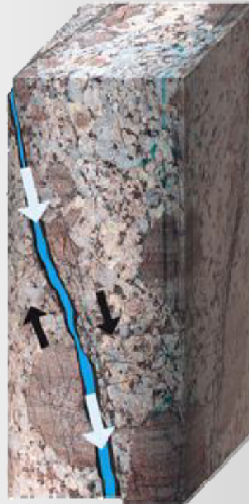
Fracture aperture during stimulation (seismic event)
