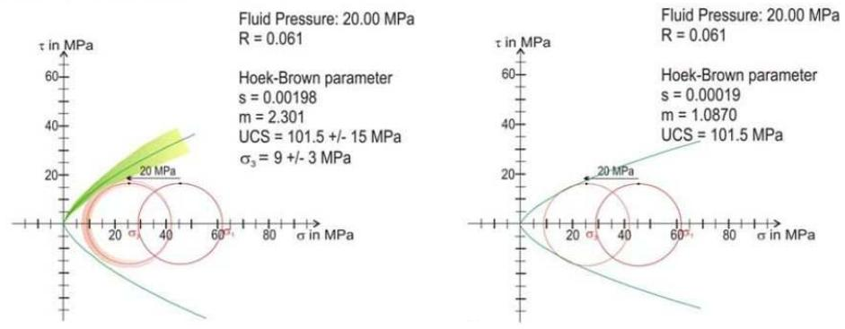
Distribution of seismicity fits orientation of F28 fault. Mohr circle diagrams show reactivation during stimulation. The stereo plot shows the slip tendency of recorded microseisms.
