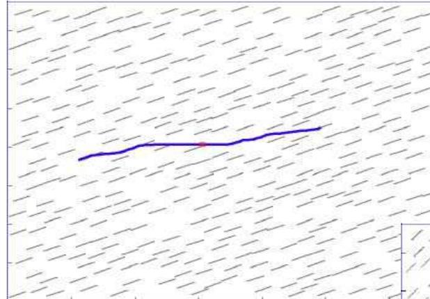
*No fracture initiation with fractures oriented at 30° from max horizontal stress*
