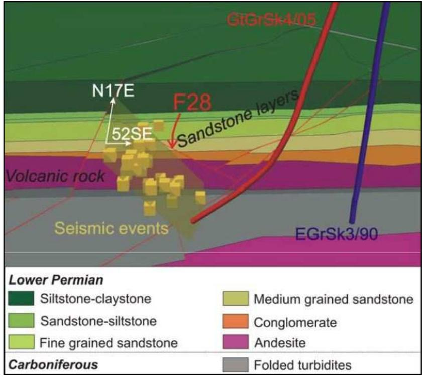
Stress state and failure
