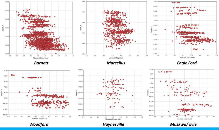
Moment magnitude ->Seismic moment -> f (shear modulus, fault plane slip distance, slip area)
