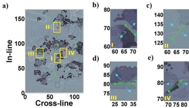
**Figure 7** (a) integrated display of FZI; (b, c, d & e) stress gradient (lighter arrows) and discontinuity boundary (darker arrows) overlaid on the FZI attribute [32].
