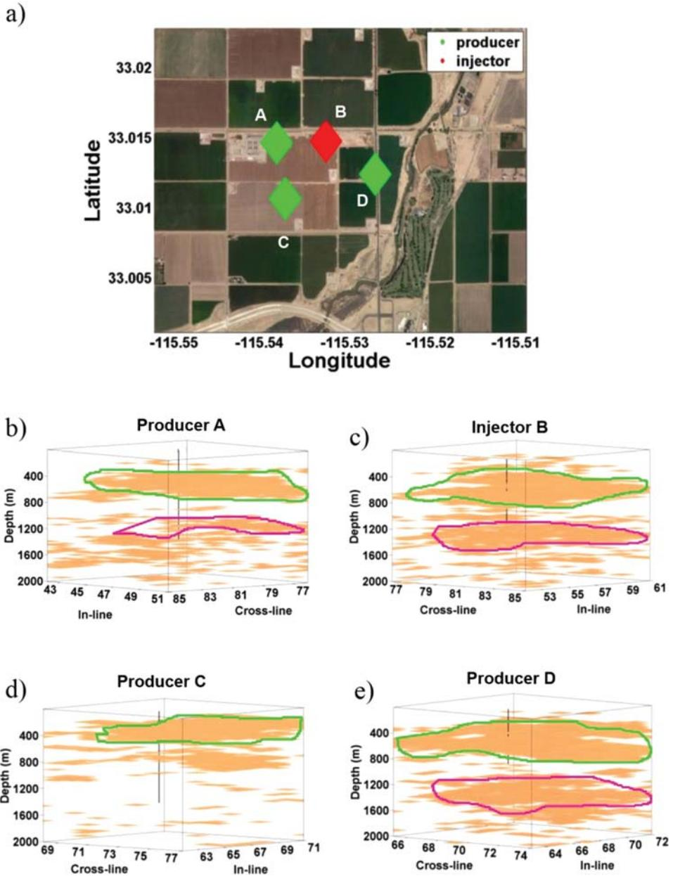
Figure 6 (a) location map of the production and injection wells; (b, c, d, and e) show the FZI attribute for producers A, C, and D as well as the injector B [32].
