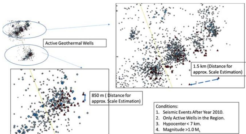
**Figure 9** Mapped Earthquakes since 2010 with the active geothermal wells (generated for this article [45]).
