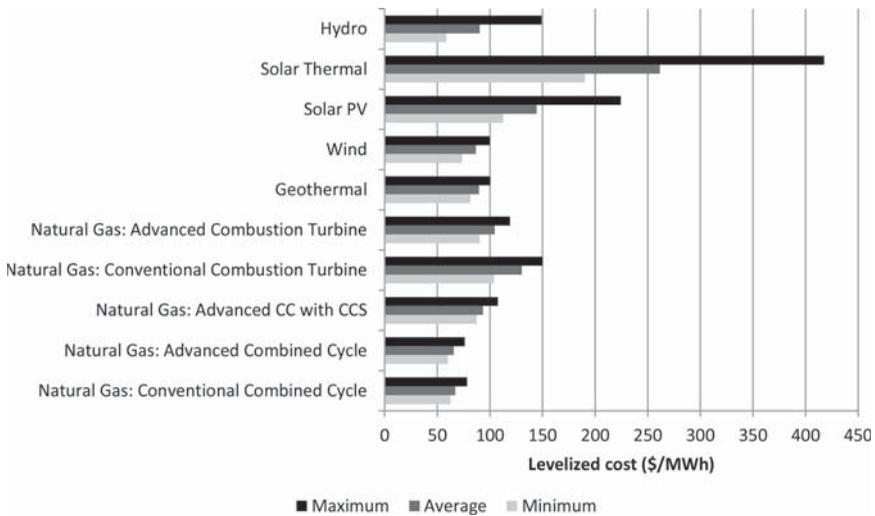
**Figure 5** Predicted levelized costs, by technology, expected for generation brought online in the year 2018 [40].
